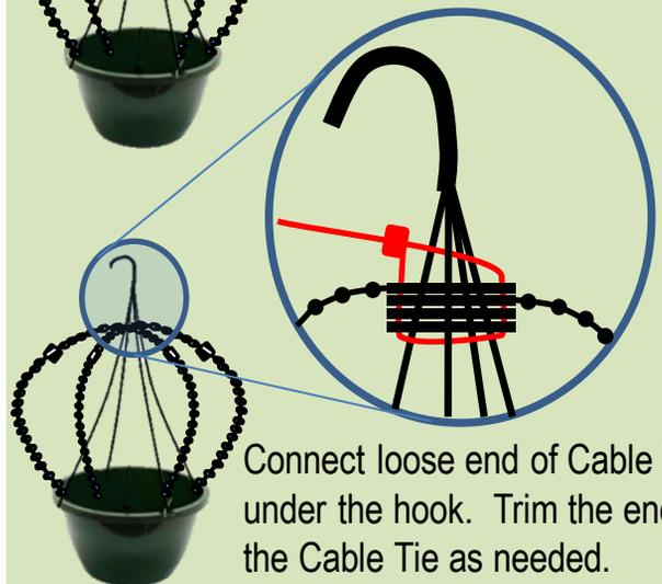
Connect loose end of Cable Tie under the hook. Trim the end of the Cable Tie as needed.
