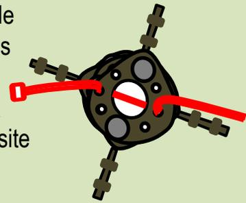
Push the top of the trellis down to expose the wire (or chain) hanger strands through the hole at the top.
