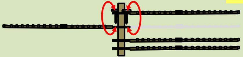
Align the small holes with the Pins and pinch together
